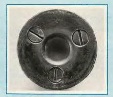
Heads of tie rods which hold baffles.
